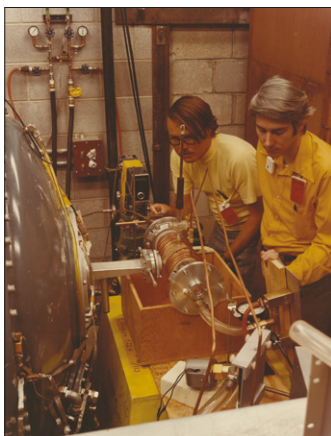
Silfvast and colleague Obert Wood attempting to pump a lead vapour laser with a Febatron at Sandia Labs in Albuquerque, NM in 1974.
