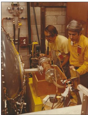
Silfvast and colleague Obert Wood attempting to pump a lead vapour laser with a Febatron at Sandia Labs in Albuquerque, NM in 1974.
