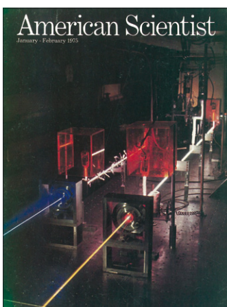
An American Scientist cover showing Silfvast's laboratory with a He-Cd laser and a He-Se laser.
