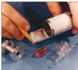
The first ruby laser is disassembled.
