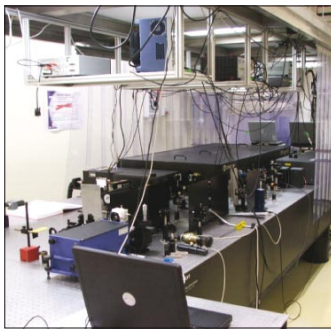
A high-energy Ti:Sapphire-based ultrafast system for photoinjector applications in the laboratory for lasers and optical fibres at Elletra, Sincrotrone-Trieste, Italy.
